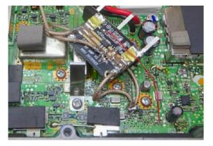
Cut PCB track between C271 and F1271. Connect LNA input to C271. Output of amplifier to F1271. +5V Rx connected at the junction of C274, C275, R271.
