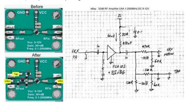
A low cost eBay LNA 0.05-4G NF=0.6dB RF Amplifier Ultra-Low Noise High Linearity FM HF VHF/UHF, is modified to split the receiver RF into two paths. The Vcc series resistor selected to power the LNA from 5V. Two simple attenuators split the amplifier output. One feeds the receiver preamp and one is fed to a rear panel SMA.
