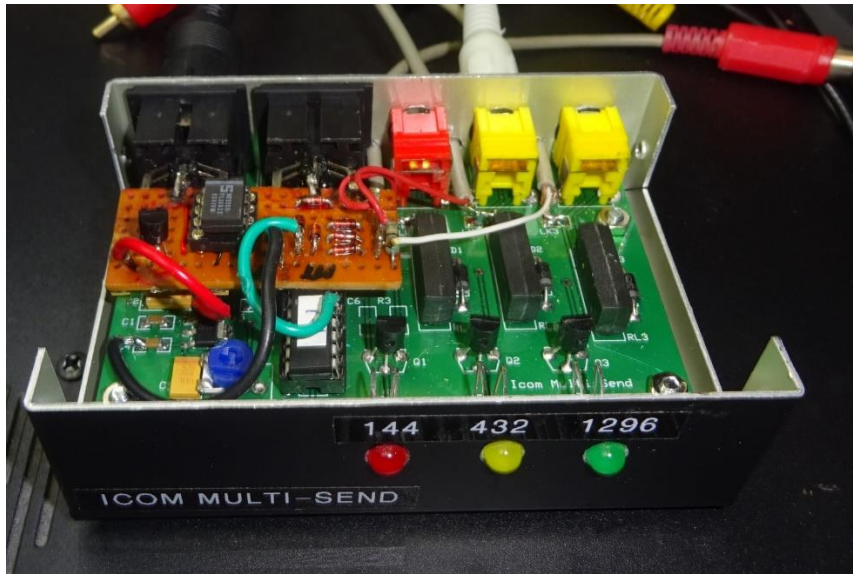
Figure 8 - ALC preconditioner and combiner installed in Icom MultiSend
