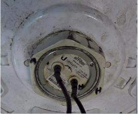
New slots allow the dipole assembly to be rotated 45° clockwise. Reassembly provides horizontal or vertical polarization. Note and mark the polarization on the rear of the dipole assembly.
