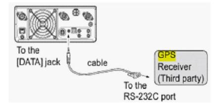
Mono plugs may be used where GPS NMEA sentences are being sent to radio from GPS receiver.
