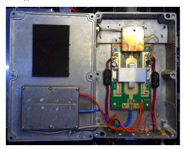
The RF deck is mounted on a large air cooled heatsink and shielded in a diecast aluminium enclosure. The enclosure also contains the driver and the output reflectometer. RF input is via a SMA female flange jack and the output through a N female flange jack. Power supply feeds and SWR monitoring signals are connected through feed through capacitors.
