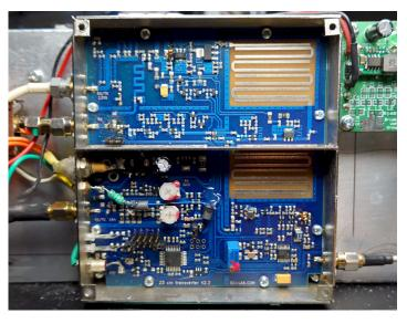
The output of the transverter is 1 W approx. for 5W IF drive.
