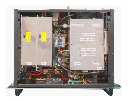
A second DC-DC down-converter operating from 24V provides 12V current limited to 1A for a masthead low noise amplifier (MH LNA) via a bias-T between the output antenna changeover relay and the rear RF output connector. A rear panel switch enables the MH LNA and isolates the bias-T supply for testing and when a MH LNA is not used.
