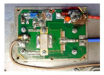
The driver, with a supply of 12Vdc, produces over 5W to drive for the final power amplifier. The supply voltage is limited to ensure the driver cannot damage the power amplifier input. The driver may draw up to 1A.
