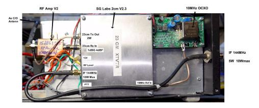
As the modified transverter had inadequate receive gain and relatively poor noise figure the receiver input is supplemented with a RF Amplifier V2 (PGA-103).
