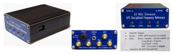
The module is based on a CTI OSC5AB02 oven-controlled crystal oscillator OCXO, square wave, operating at 5V. The inherent OCXO has a warm-up time is less than 2 mins and stability is better han 10 ppb (±0.1Hz) at 0°C to 45°C. Phase noise is -80dBc/Hz@1Hz, -120dBc/Hz@10Hz, -140dBc/Hz@100Hz, -145dBc/Hz@ 1kHz, -150dBc/Hz.
