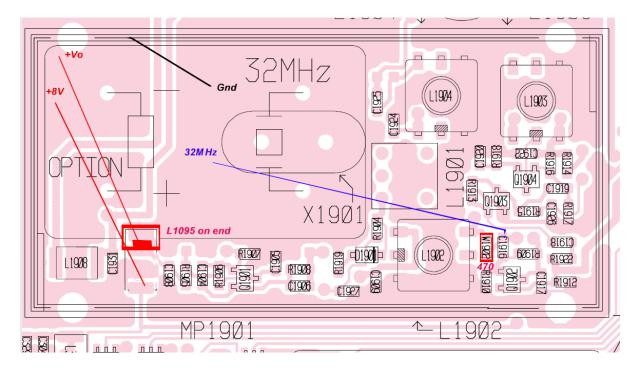
Power for the RefGen is drawn from the +8V supply to the reference oscillator. The controlled +8V for the oscillator is fed to the radio reference oscillator. A feed-point for the 32MHz reference from the RefGen module is the junction of W1902 and C1916. To increase the impedance at this feed point, W1902 (OR 0603 resistor) is replaced with a 470R 0603 resistor. Ground for the RefGen is provided by pigtails soldered to the shield of the 32MHz reference oscillator.
