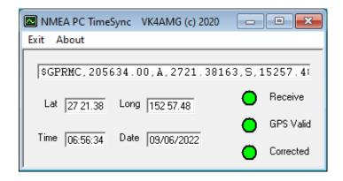
If the GPS receiver is sending NMEA RMC messages the 'Receive' LED will flash Red every second. When the GPS receiver reports the GPS is receiving valid position and time fix, the 'GPS Valid' LED will light green. The GPS NMEA RMC message will be displayed together with the date and time and the latitude and longitude. At the 25<sup>th</sup> and 55<sup>th</sup> GPS second, a correction will be applied to synchronise the PC time.
