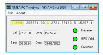
\$GPRMC message is not displayed in text box. Check GPS receiver baud rate is correctly configured / selected in the application. 4800 baud is default NMEA but 9600 is becoming more common. Brisbane VHF Group GPSD-1 is configured for 9600 baud.
