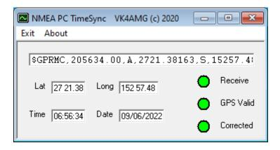
A GPS receiver may provide many common messages (refer <u>NMEA-0183 messages: Overview</u> (<u>trimble.com</u>)) The NMEA RMC sentence (refer <u>NMEA-0183 message: RMC (trimble.com</u>)) is a NMEA-0183 message providing Position, velocity, and time.
