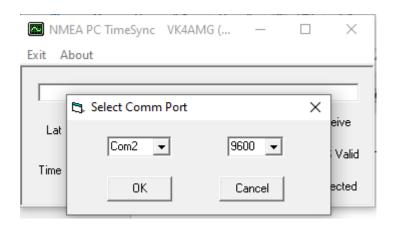
If an alternative comm port and / or baud rate is required, select them from the Pull-down lists. Click 'OK'. If no action is taken the 'Select Comm Port' dialog will close after a short delay and the application will run. Com1 through Com9 only allowed.
