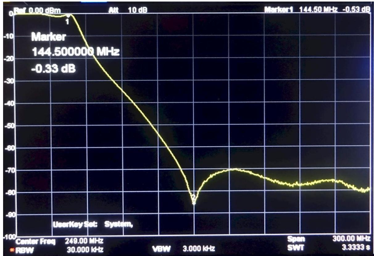
The result is a low loss LPF with excellent attenuation at the 144MHz harmonic frequencies.
