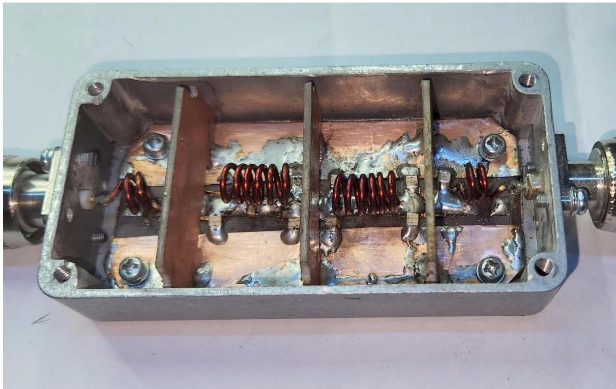
This filter is built in a 1590B diecast aluminium enclosure. Double sided PTFE board from Larcan amplifier splitter combiner was used to support the components. Copper sheet was fixed either side of the component mounting strip. The copper was soldered to the ground plane side of the board and then folded over the edges of the board. Short pigtails pinned the top copper sheet to the ground plane at multiple points.
